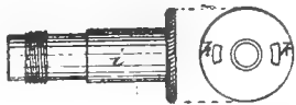
Fig. 8. Side view of the sleeve i and front view of beveled slots k k.
